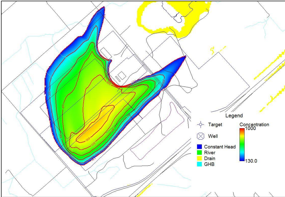
Figure 34: Maximum Simulated Concentration with New Landfill; Chloride Concentrations greater than 130 mg/L, Year 2064, Layer 3
